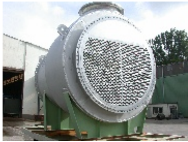
Fa. Ineos Phenol Werkstoff= 1.4571 \text{Ø}=2.100 / L= 4.630 / \text{kg}= 21.100
